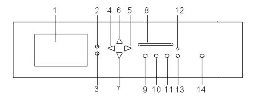
1.LCD display interface: display various parameters during commissioning, and display alarm records and number of people passing the test.
